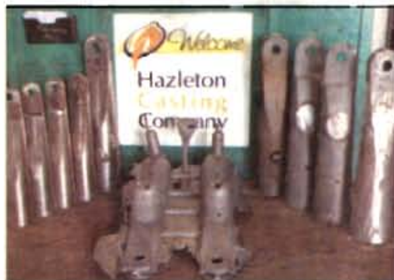
From core box, center, to raw supports at right, and the finished product, left, a display shows stages of supports made at Hazleton Casting.
